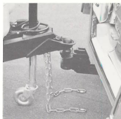
2. Lower trailer, insert safety pin.
