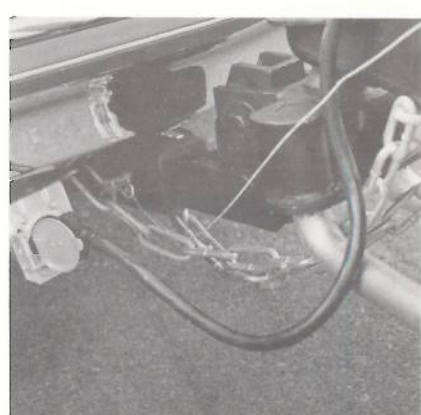
8. Connect break-away switch cable.
