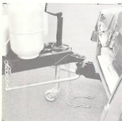
3. Raise trailer and car, attach bars.
