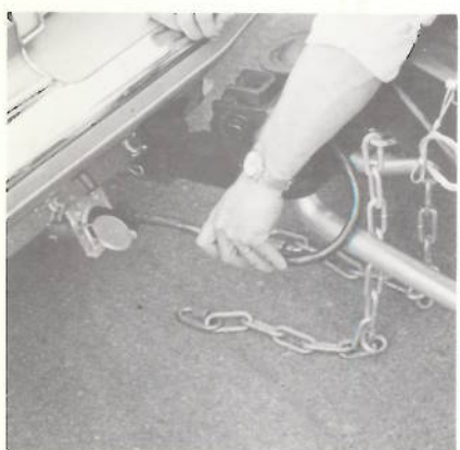
6. Hook up electrical connector.
