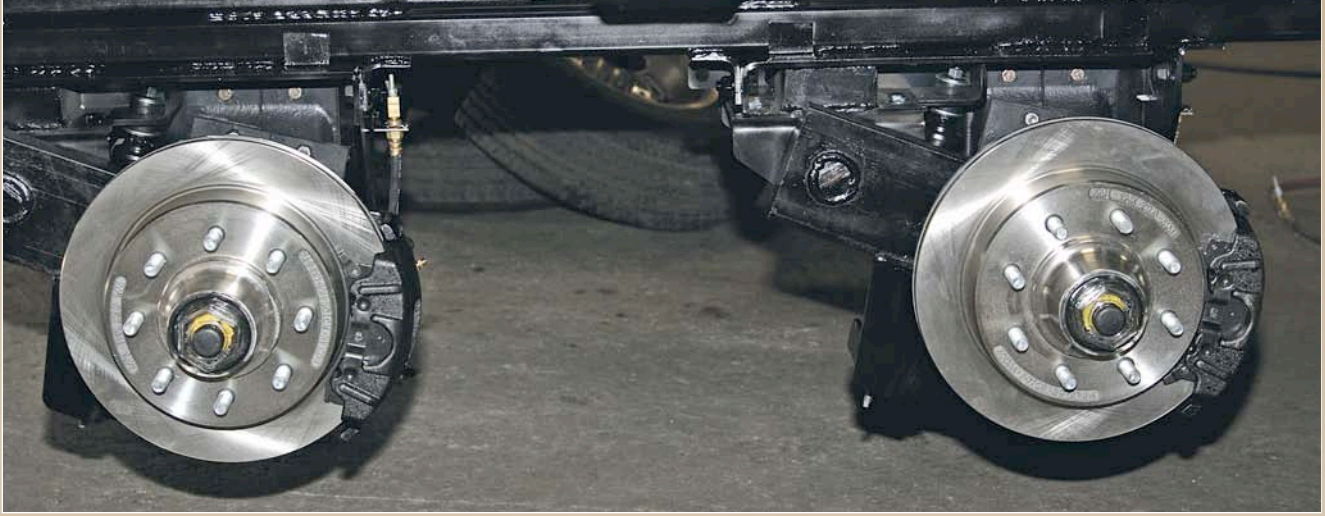
The completed MOR/ryde IS Suspension System upgrade with Kodiak Disc Brakes. Next up: tires, wheels, and laser alignment.
